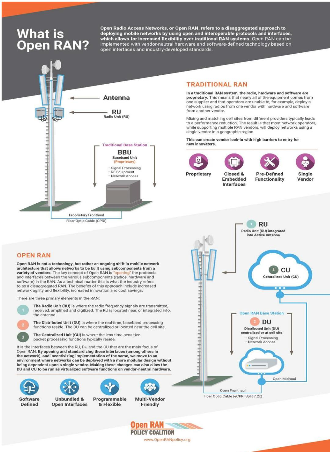
Originally defined by 3GPP to facilitate Ultra Reliable Low Latency Communication and Enhanced Mobile Broadband requirements, specifications in 3GPP Release 15 divided the
